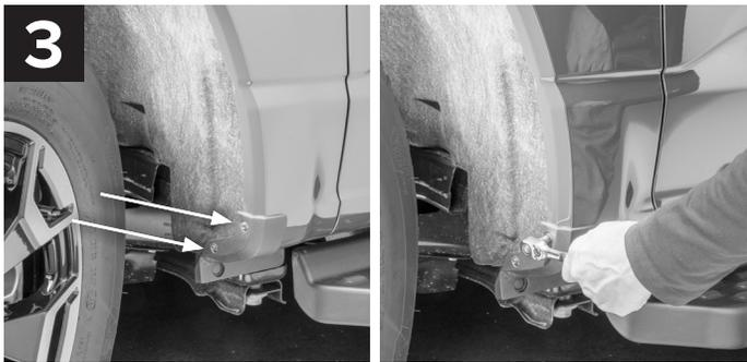
Locate the (2) two hex head screws at the inner fender as indicated. Using a ratchet and appropriate socket, remove these screws. They will be reused.
