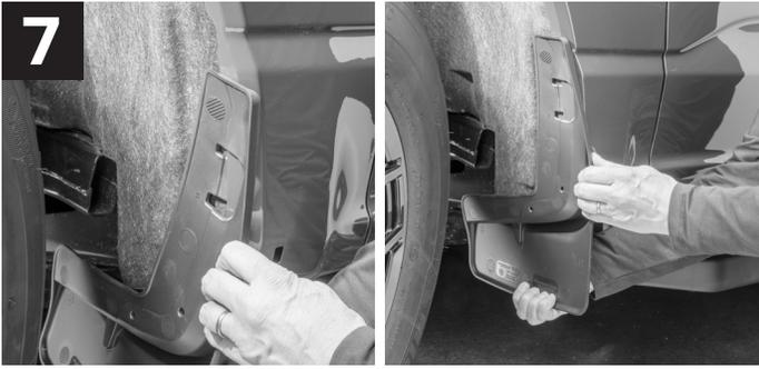
Using the MudFlap marked “LH,” place it up to the fender while sliding the tab underneath the fender lip. Then align with the corresponding holes in the vehicle.
