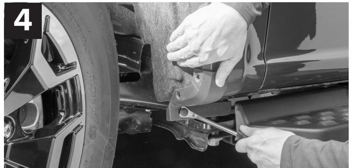
Locate the (1) one plastic fastener in the factory chip guard. Using a trim clip remover, remove this fastener. It will not be reused.
