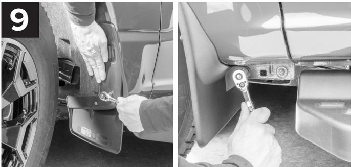
While firmly pressing the MudFlap up to the fender, fully tighten the (2) two hex head screws and (1) bolt.
