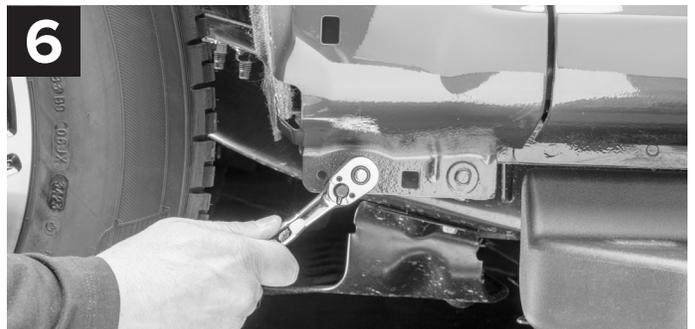
Locate and remove the (1) one front factory bolt using a ratchet and appropriate socket. It will be reused.
