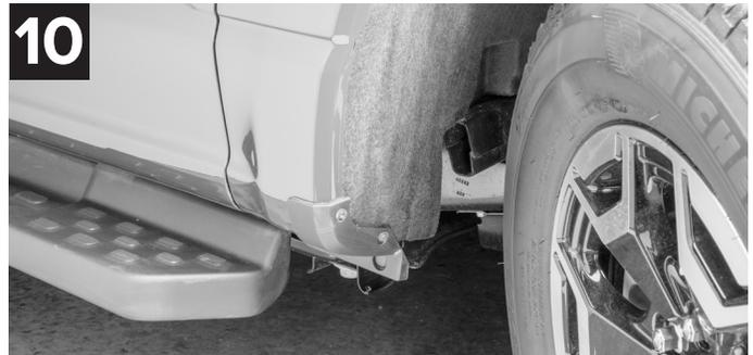
Install the passenger side MudFlap marked “RH” with the wheels turned fully to the right, repeating Steps 3-9.
