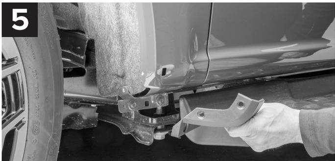
Remove the factory chip guard by pulling it out from the fender. It will not be reused.
