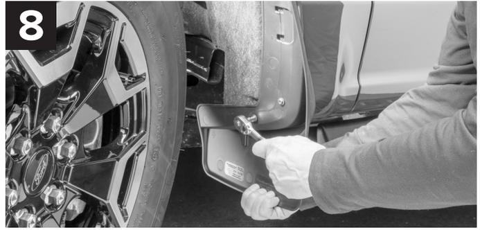
Re-install the previously removed (2) hex head screws and (1) bolt to a loose fit.
