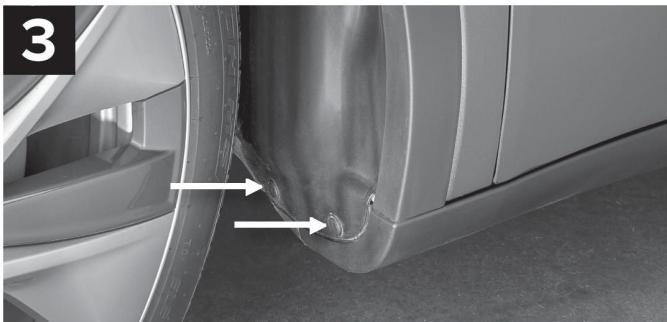
Locate the (2) two factory plastic fasteners at the inner fender as indicated.
