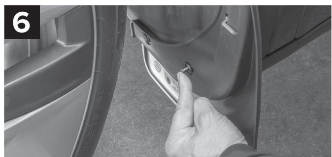
Take (2) two supplied plastic fasteners and install them by inserting them through the MudFlap holes and inner fender, then fully depress the head to lock them in place.
