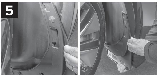
Using the MudFlap marked "LH", place it up to the fender and engage the tab behind the fender lip. Then slide it into place where it aligns with the corresponding fastener holes and is tight against the inner fender.
