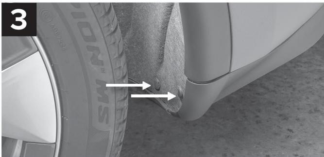
Locate the (2) two factory plastic fasteners at the inner fender as indicated.
