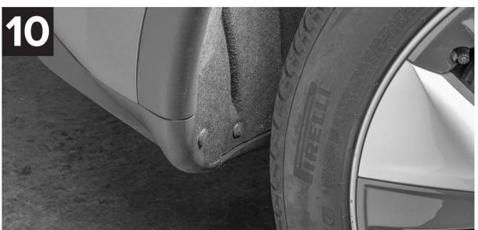
Install the passenger side MudFlap marked "RH," repeating Steps 3-9.
