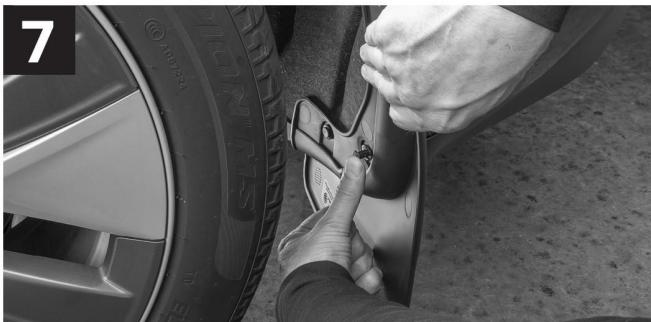
Take (2) two supplied plastic fasteners and install them by inserting through the MudFlap holes and inner fender, then fully depress the head to lock them in place.
