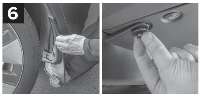
Using the MudFlap marked "LH," place it up to the fender and align with the corresponding holes. Then, loosely reinstall the screw from Step 5.
