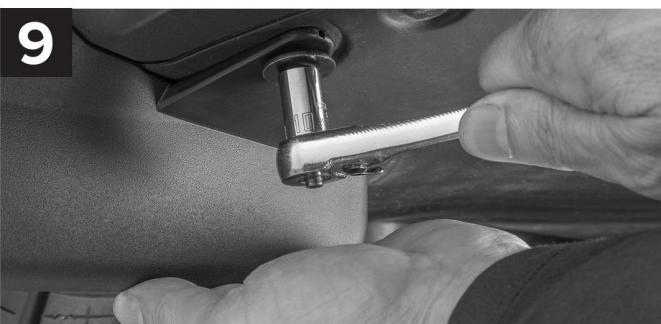
Fully tighten the screw on the underside of the fender.
