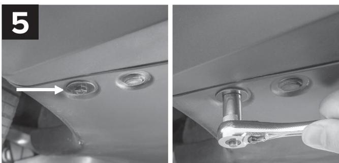
Locate the (1) one factory screw on the underside of the fender as indicated. Using a ratchet and appropriate socket, remove this screw. It will be reused.
