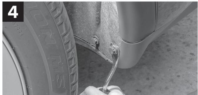
Using a trim clip remover, remove the (2) two factory plastic fasteners at the inner fender. Pry the head up and then the base out of the fender. They will not be reused.
