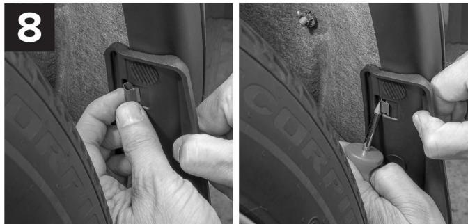
Install (1) one supplied U-Clip by placing it where it clamps around the MudFlap and fender lip, then push it into place with a flat blade screwdriver.
